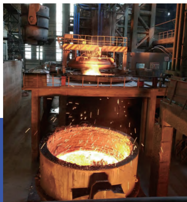
260t VD Vacuum Refining Furnace
