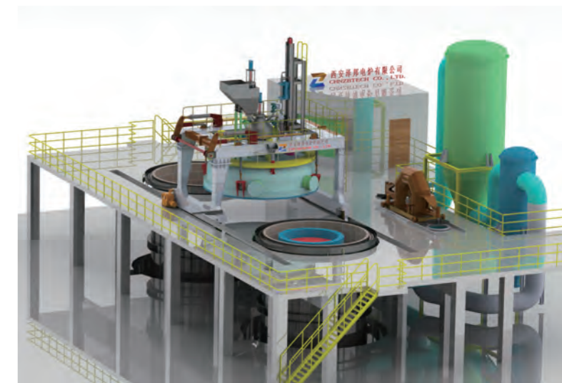
Overall Layout Of 180tVOD Vacuum Refining Furnace
