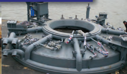
Water-cooled roof of EAF
